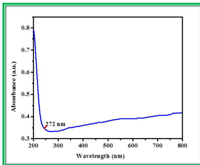
**Figure 3 (a): UV-Visible Spectrum of NiO Nanoparticles**
