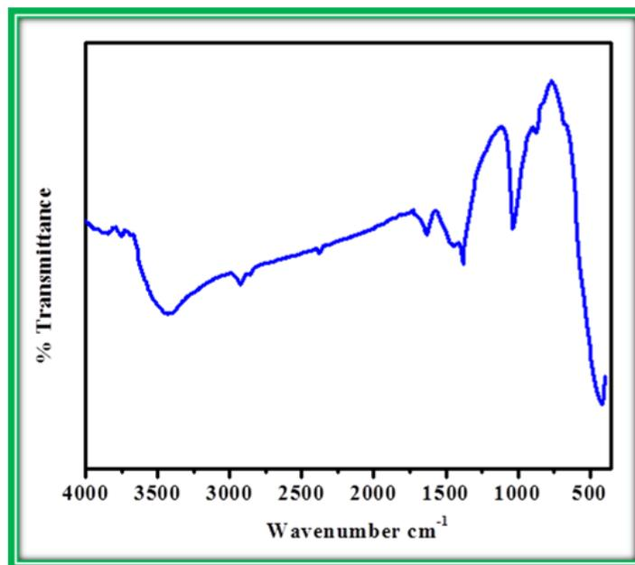
**Figure 2: FTIR spectrum of NiO nanoparticles**
