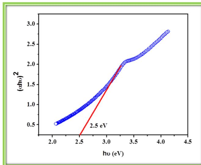
**Figure 3 (b): Band Spectrum of NiO Nanoparticles**
